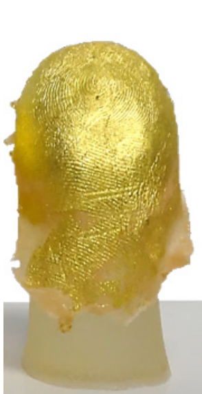
Figure 1: Conductive artifact – latex face paint with edible gold leaf coating
