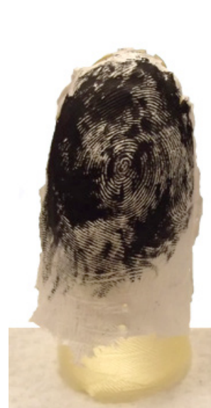
Figure 3: Conductive artifact – acrylic paint with Bare Conductive Paint coating
