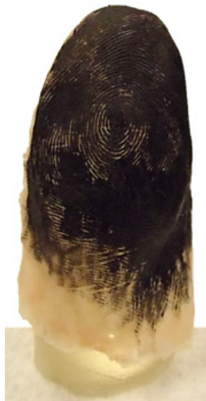
Figure 2: Conductive artifact – latex face paint with Bare Conductive Paint coating
