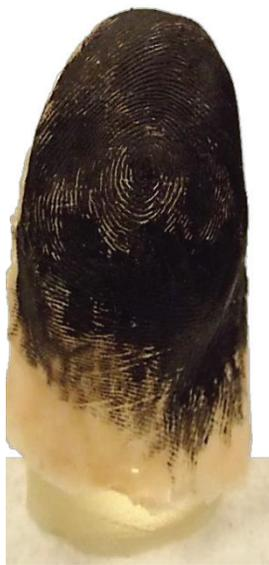
*Figure 2: Conductive artifact - latex face paint with Bare Conductive Paint coating*
