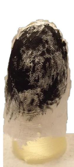
*Figure 3: Conductive artifact - acrylic paint with Bare Conductive Paint coating*
